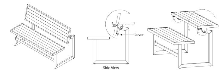
**Note:** To convert from bench to table and vice versa, press the lever in the direction of the arrows (upwards). This operation can be done on one side only.
